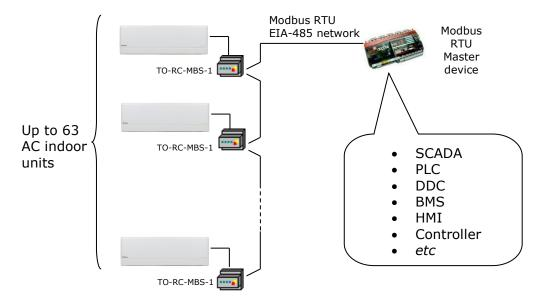
The TO-RC-MBS-1 interface allows a complete and natural integration of **Toshiba** air conditioners into Modbus RTU (EIA-485) networks.
