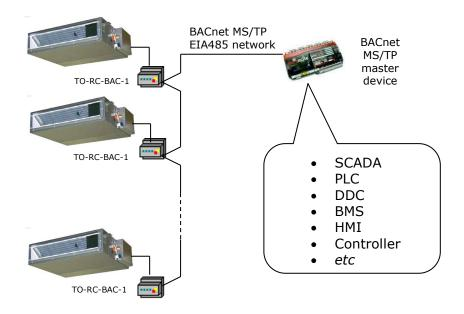
The TO-RC-BAC-1 interface allows a complete and natural integration of *Toshiba* air conditioners into either BACnet IP or MS/TP networks. Compatible with the VRF line models commercialized by TOSHIBA
